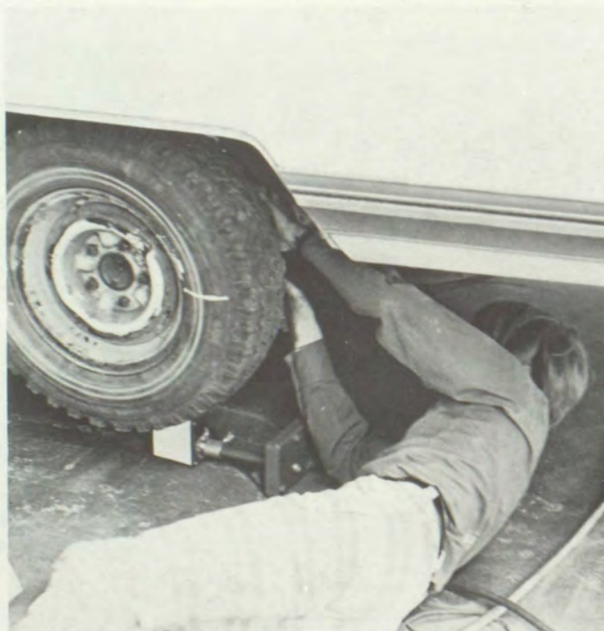
During his auto mechanics class, Dave Beer applies a strobe balancer to a wheel.
